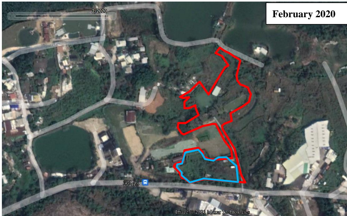
Figure 1-2 A part of the site and the pervious application A/YL-LFS/401 (marked in blue) has been subject to land formation and vegetation clearance. It is suspected that this is a case of “destroy first, build later” (Source: Google Earth) (the application site marked in red)
